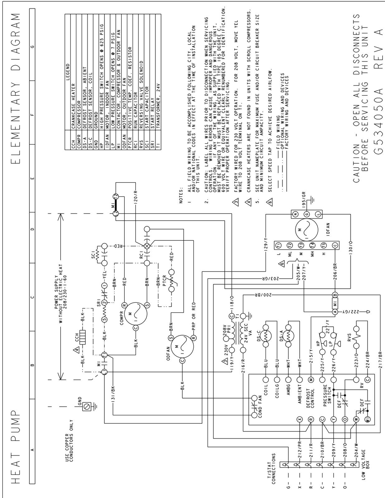
UQ036, 048 and 060 Typical Heat Pump 208/230-3-60 volt Wiring Diagram
